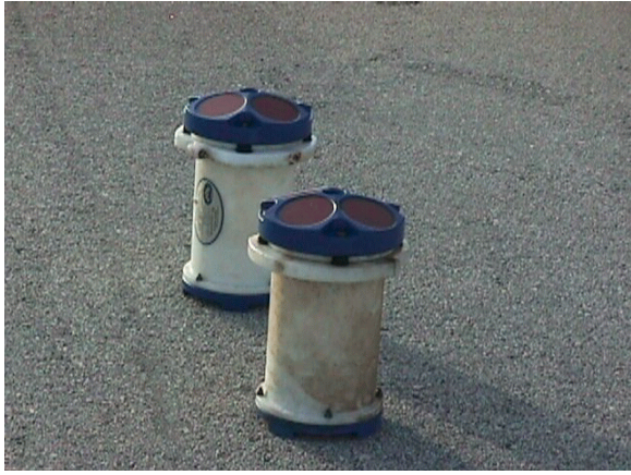
Two of the RDI Workhorse ADCPs used for the survey.
