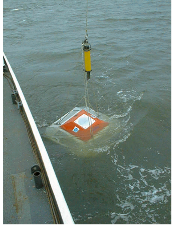
Deployment of a bottom-mount over the side of the vessel using an acoustic release and crane.
