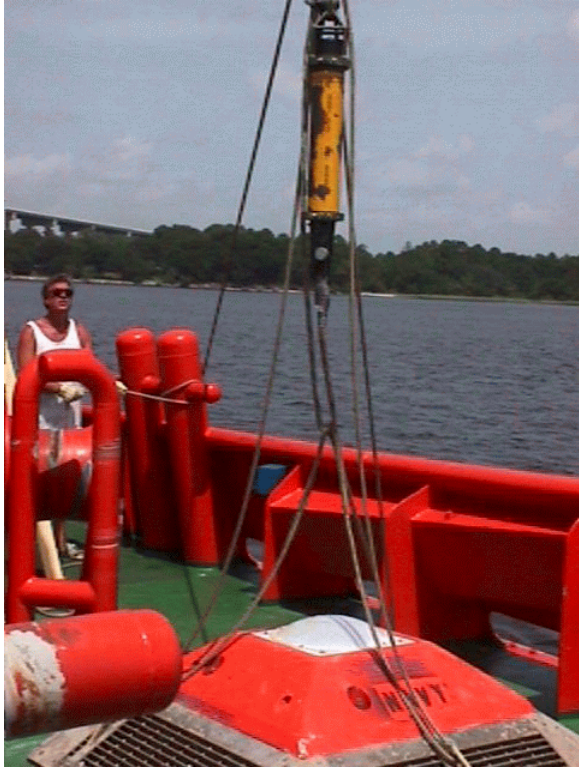
Preparing for the deployment of a bottom-mount using an acoustic release crane.
