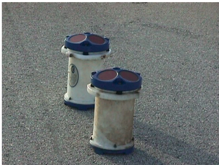
Figure 2.1 RDI Workhorse ADCPs used for this survey.
