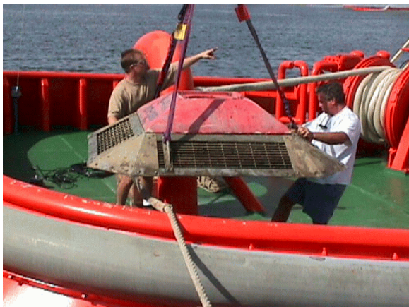
Loading a cleaned-up bottom-mount back onto the vessel, ready for re-deployment.
