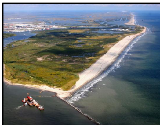
Belle Pass, Louisiana Pumpout for Caminada Headland Restoration. Photo courtesy of Weeks Marine
