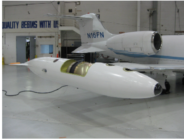
Figure 4.16: One INFLAME INSTRUMENT (IN THE GOLD COLORED HOUSING) MOUNTED IN A LEARJET WING TIP POD JUST PRIOR TO FLIGHT DEMONSTRATION IN JANUARY 2010.
