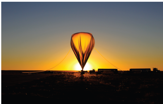
(a) The high-altitude balloon that carried the HySICS instrument to the outermost part of Earth atmosphere was inflated with helium.
