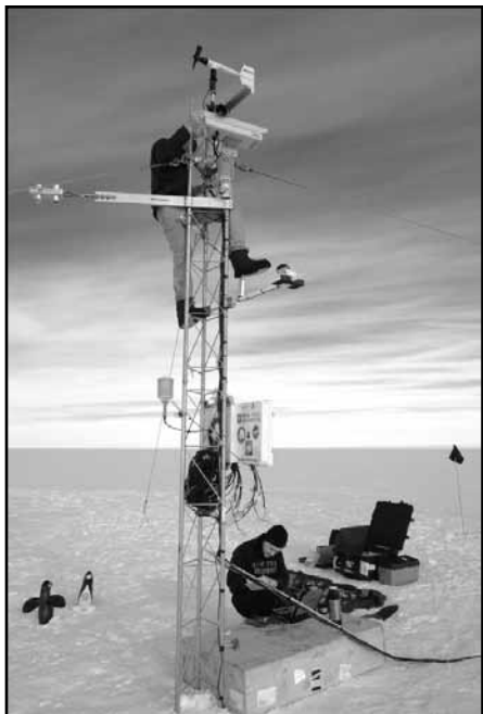
Weather instruments and Global positioning systems are placed on the ice near Pine Island Glacier.
