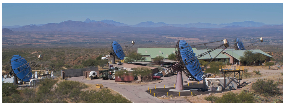
FIGURE 7.10 ACTA would be, like the pictured VERITAS (Very Energetic Radiation Imaging Telescope Array System), an array of Čerenkov telescopes used to detect very high energy (TeV) gamma rays emanating from astrophysical sources. The proposed ACTA telescope would be a larger-scale international version of this facility and similar ones located in Namibia and the Canary Islands that would increase the sensitivity by roughly an order of magnitude. SOURCE: Image courtesy of Steve Criswell, SAO.
