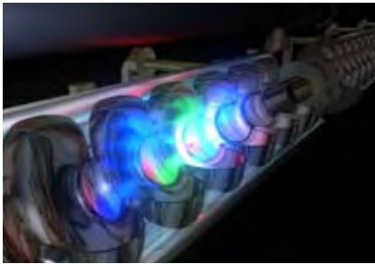
Computer animation of the field inside a superconducting accelerator resonator Image courtesy of DESY
