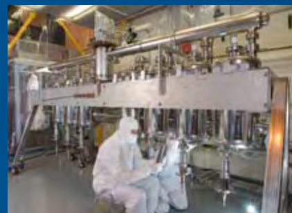
Assembly of a superconducting accelerator section for production of ion beams Photo courtesy of J. Nolen, Argonne National Laboratory
