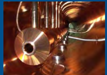
View into the linac portion of the Spallation Neutron Source at Oak Ridge National Laboratory Photo courtesy of Oak Ridge National Laboratory
