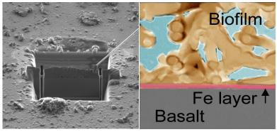
Focused ion beam technology allows preparation of a precise crosssection into the basalt sample covered with a newly formed iron layer and biofilm. A thin section is used for imaging and analyses by transmission electron microscopy.
