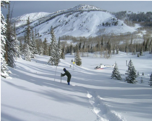
Manual measurement of snowpack at a snow course in Utah.
