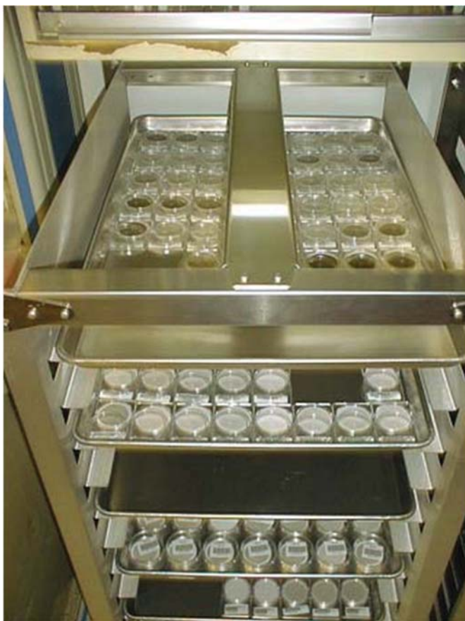
Figure 10.1 Filters equilibrating on conditioning trays
