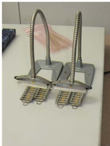
Figure 9.4: ^{210}\text{Po} Anti-static strips & gooseneck holders
