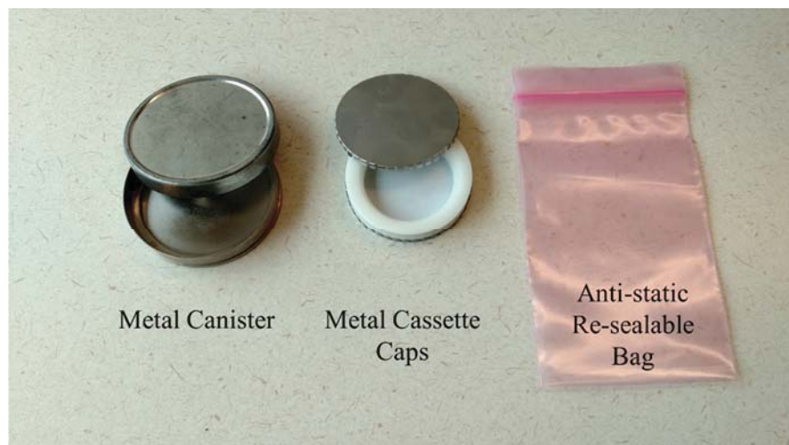
Figure 4.2 Example equipment for transporting filter cassettes
