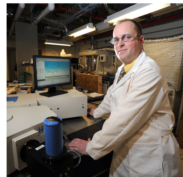
Leigh Martin performs fluorescence experiments to monitor binding of lanthanides to the magnetic nanoparticles.
