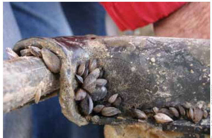
Quagga mussels infest this piece of marine equipment, pulled from Lake Mead, Nevada.
