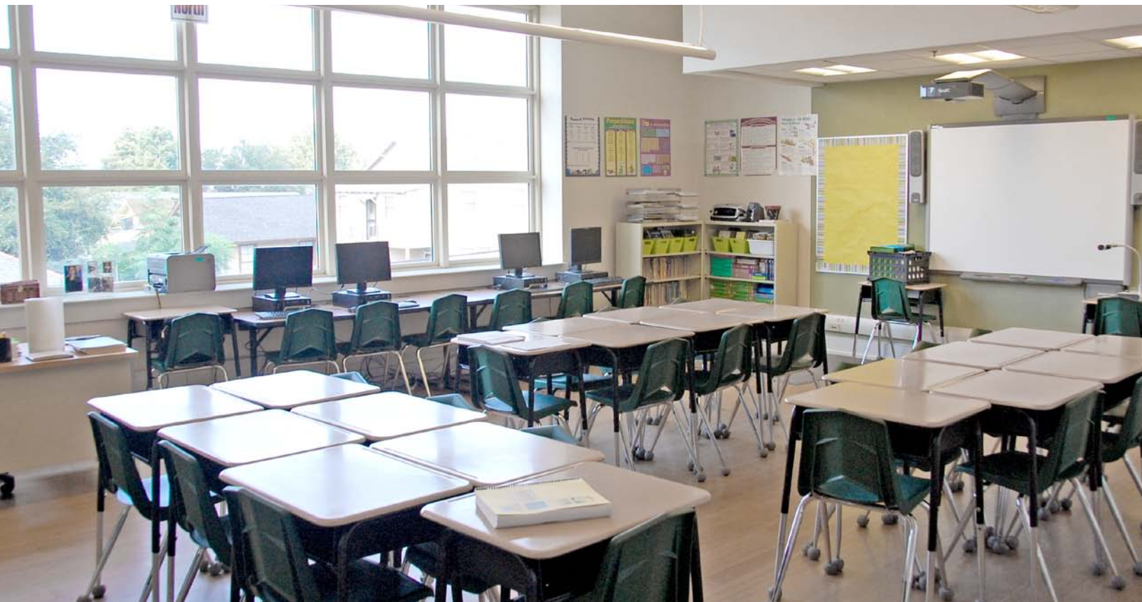
Andrew H. Wilson Elementary School's design team partnered with a daylighting leader in the United States to incorporate innovative shading devices, interior and exterior shelves, overhangs, and fabric baffles to provide daylighting to classrooms. Photo by Joe Ryan, NREL/PIX 19652
