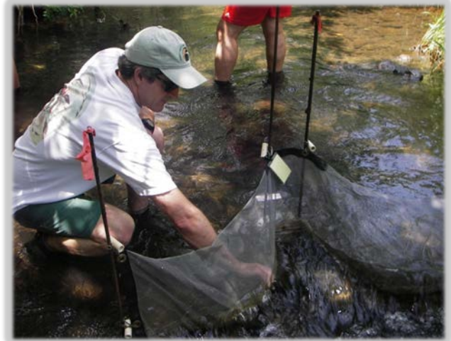
Upstream movement of fish and invertebrates is monitored using small fish traps. Credit: Paula Levin/USFWS
