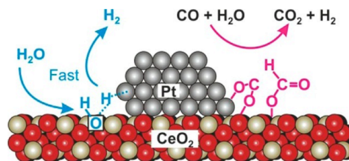
Fig. 2: Water-gas shift reaction at a Pt/CeO 2 interface.
