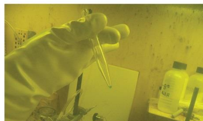
The green dot at the bottom of the glass vial is a solution containing 22 milligrams of ultra-pure Bk-249 produced at ORNL's High Flux Isotope Reactor and Radiochemical Engineering Development Center at ORNL. (Source: ORNL)
