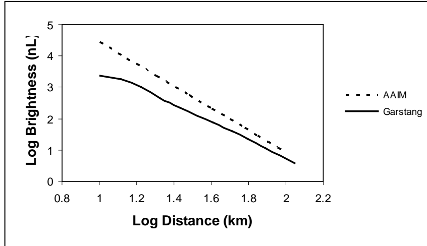
Figure 5. Sky brightness due to Denver as a function of distance for a zenith angle of zero.
