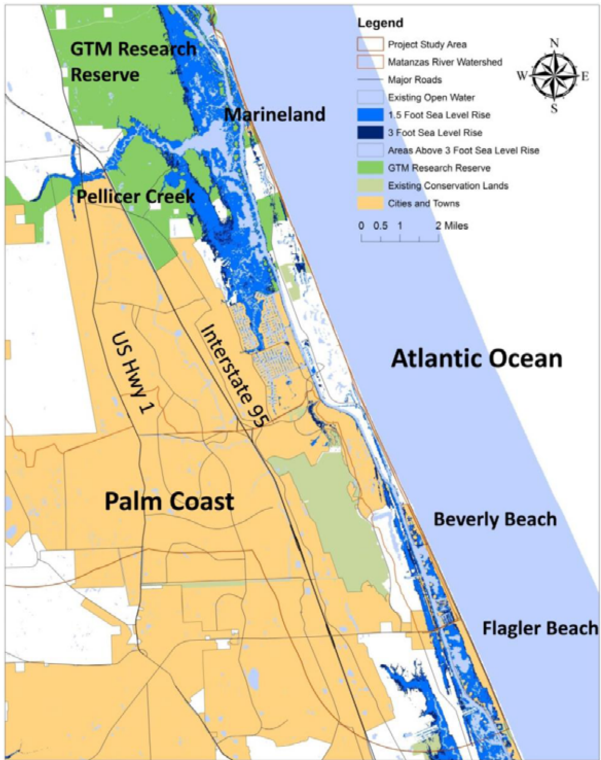
Figure 34. Inundation from 1.5 and 3 feet of sea level rise around Palm Coast
