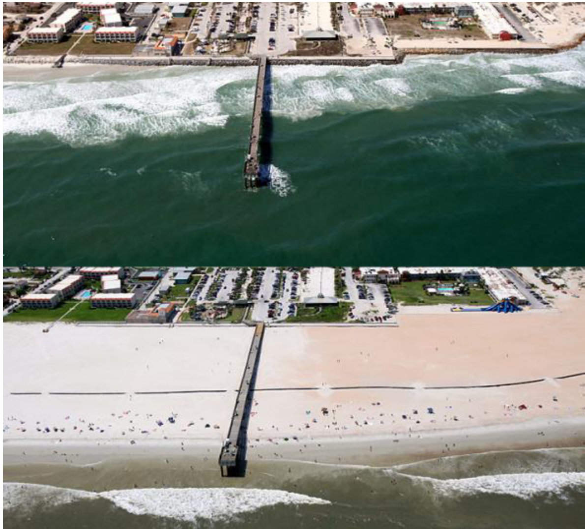
Figure 77. St. Augustine Beach, before (top photo) and after beach renourishment in 2012. Source: http://staugustine.com/news/local-news/2012-09-12/renourishment-gives-st-augustine-beach-new-look
