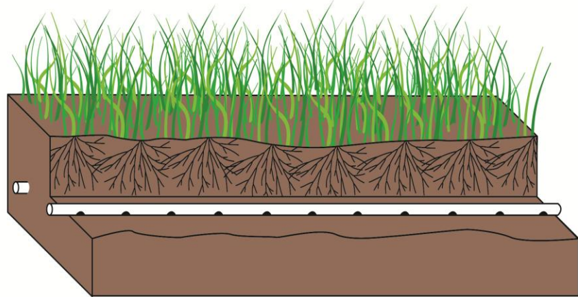
Figure 3. Cross-Section of a Shallow Pressurized Effluent Dispersal System. Other Shallow Pressurized Effluent Dispersal Systems may use chambers and other engineered materials in place of the discharge lines.
