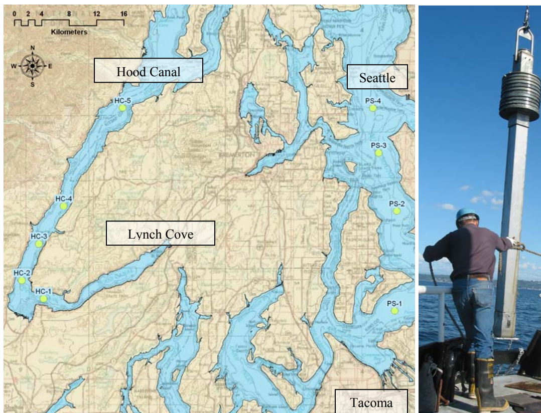
Figure 6. Sediment coring locations in central Puget Sound (PS-1 through PS-4) and Hood Canal (HC-1 through HC-5) and the Kasten corer (right).
