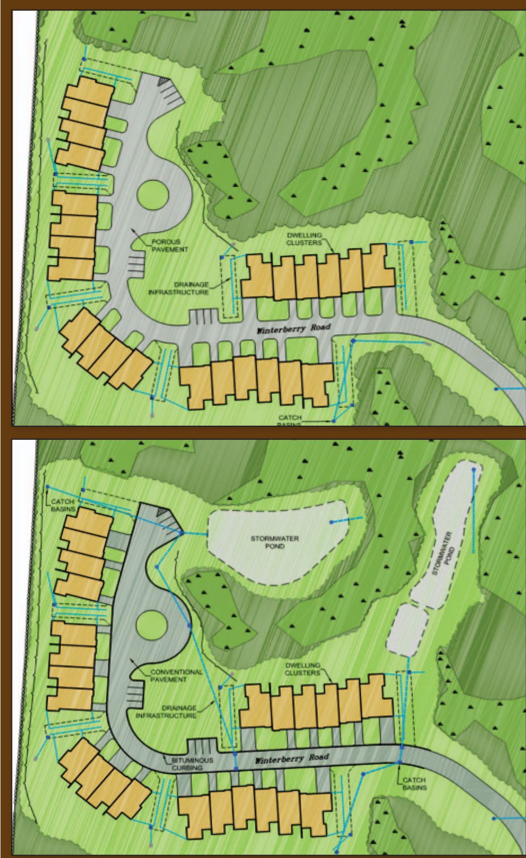
FIGURE 3-2 Comparison of Two Designs, LID Design (top) and Conventional (bottom) for Boulder Hills, Pelham, NH
