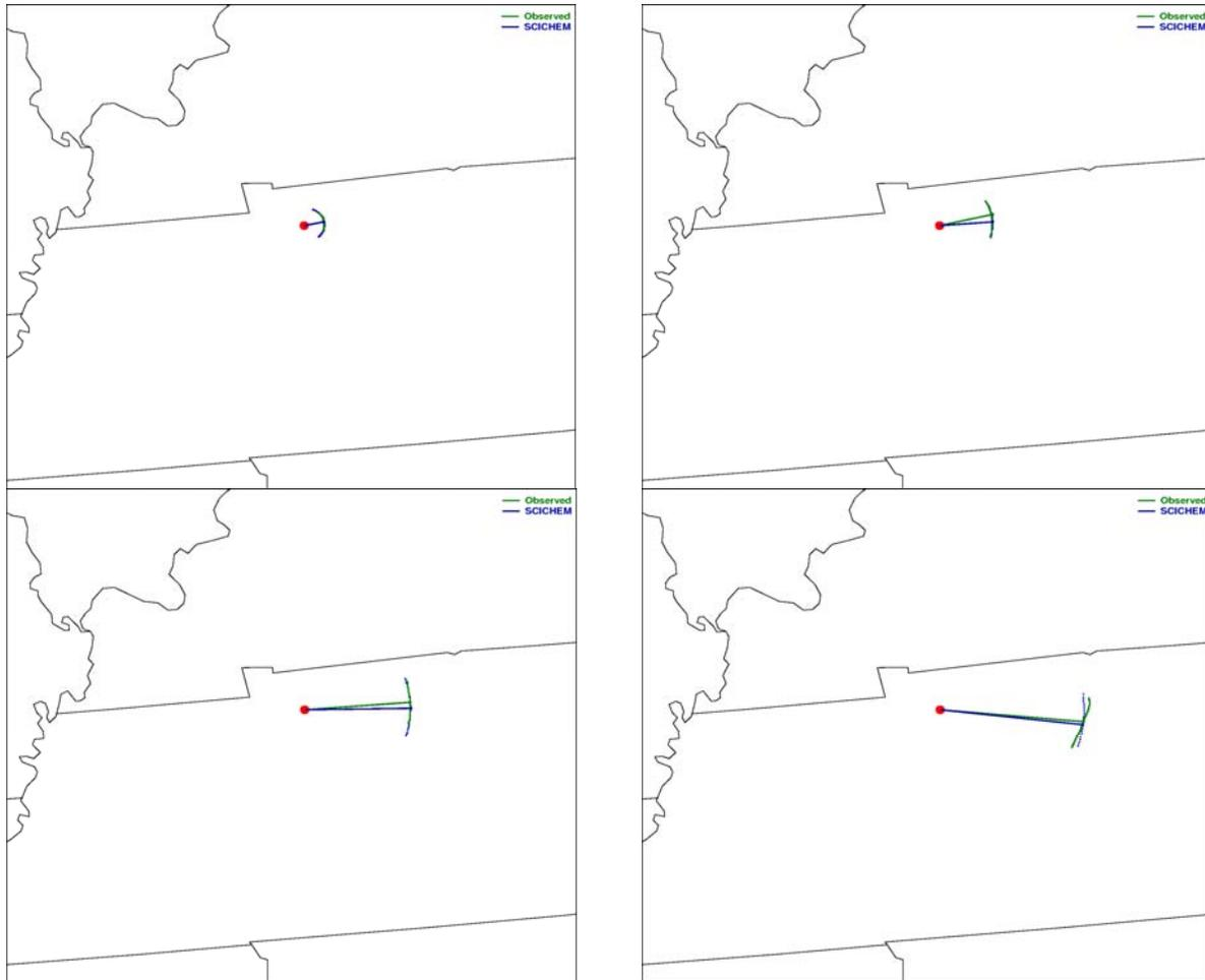
**Figure 3-1. Observed and simulated (SCICHEM) plume transport directions and plume traverses at 11 km (top left), 31 km (top right), 65 km (bottom left) and 90 km (bottom right) downwind of the Cumberland power plant on July 6, 1999. SCICHEM results are based on measured surface and upper air meteorology.**
