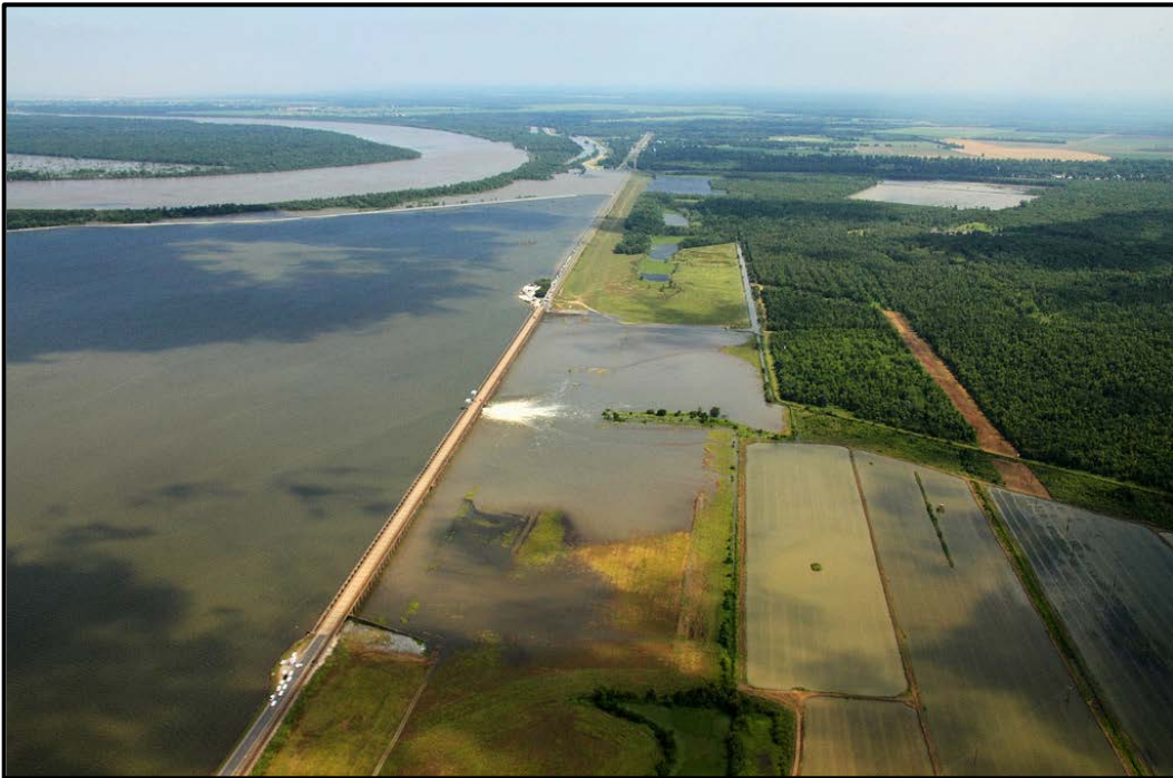
Figure A. On May 14, 2011, the U.S. Army of Corps of Engineers opened the first gate on the Morganza Floodway in Louisiana to relieve flooding on the Mississippi River. Photo Credit: U.S. Army Corps of Engineers. Available at: http://www.flickr.com/photos/30539067@N04/5722952407 .
