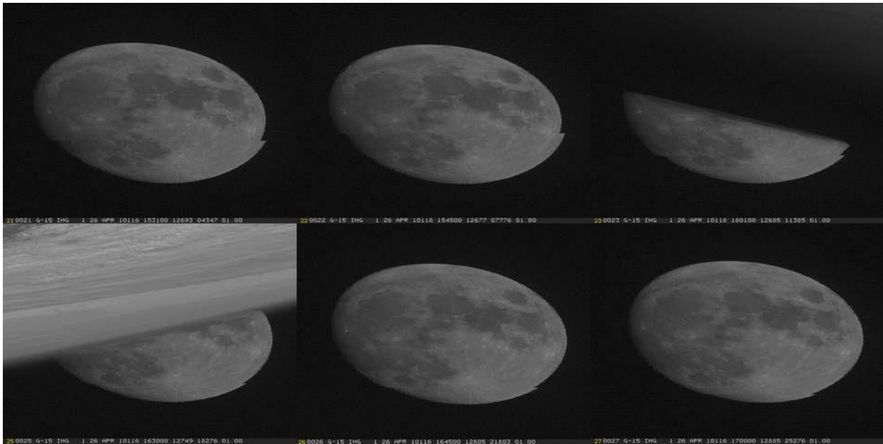
Figure 6.3: GOES-15 Imager visible ( 0.65 \mu\text{m} ) band images of the moon from various dates.
