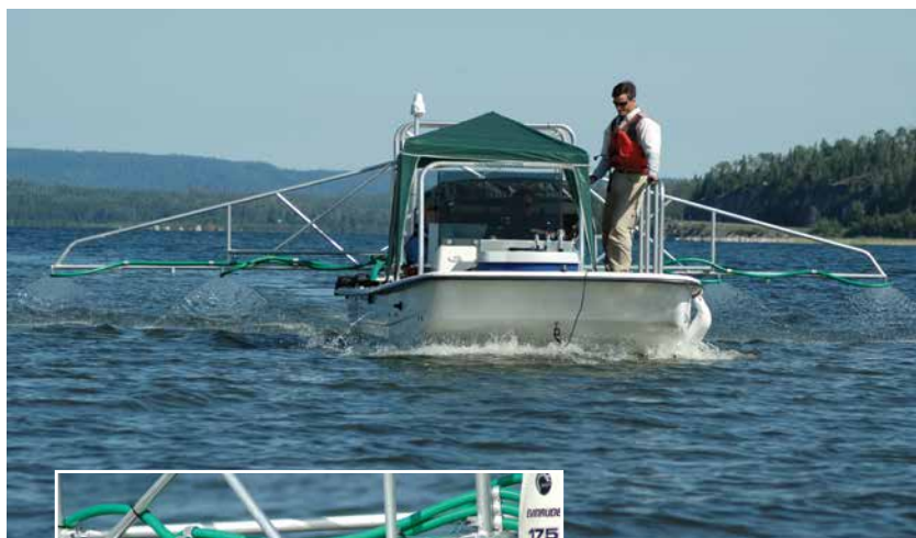
An innovative granular baylucide sprayer boat employs a high pressure spray system and GPS to effectively target lentic areas on the St. Marys River system.
