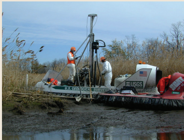
Figure H-3. Sediment coring and ground-water-quality sampling from the U.S. Geological Survey Hoverprobe in a tidal wetland of Maryland. Drilling is done by hydraulic vibracore equipment in the center of the hoverprobe craft.
