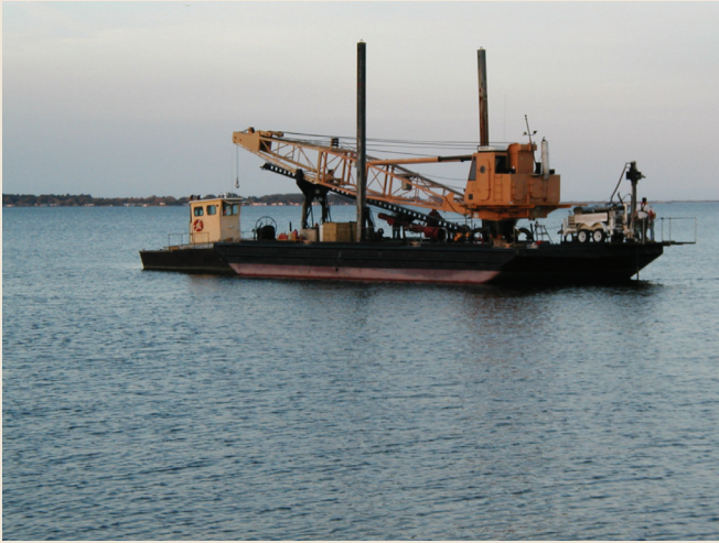
Figure H-2. State of Delaware construction barge in Indian River Bay, Delaware, with drill rig mounted on the bow of the barge.
