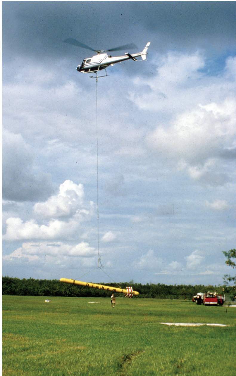
Figure 49. Helicopter and equipment “bird” collecting electromagnetic geophysical data in Everglades National Park, Florida.
