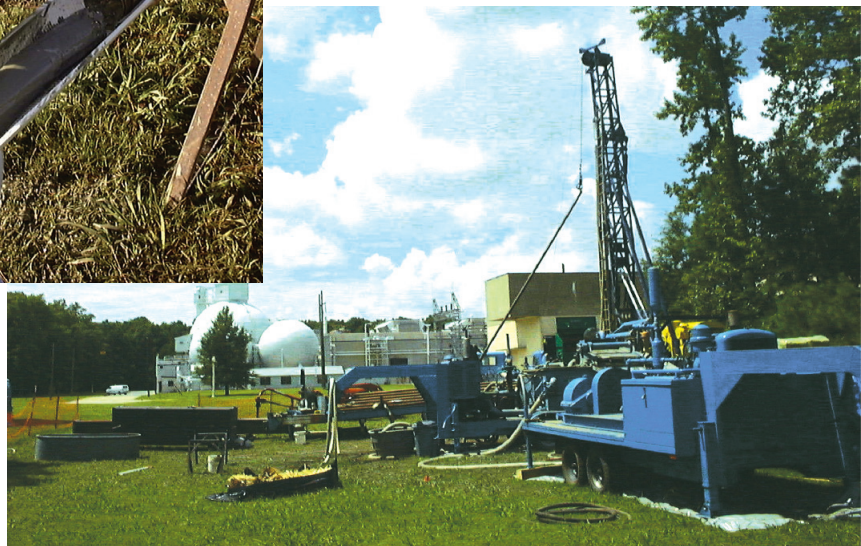
U.S. Geological Survey scientist collects sediment core at a site within the Chesapeake Bay impact crater, Hampton, Virginia, during the summer of 2000 (top). Drilling into the Chesapeake Bay impact crater at NASA Langley Research Center, Hampton, Virginia, during the summer of 2000 (bottom).
