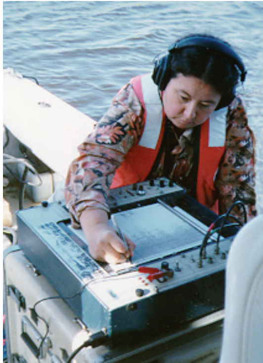
Collecting seismic-reflection data on the Neuse River, Cherry Point, North Carolina.
