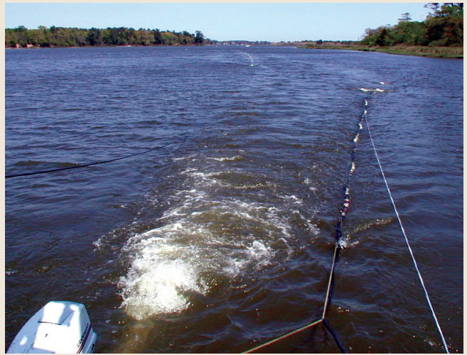
Figure H-4. Deployment of the resistivity-surveying equipment behind a small vessel in Indian River Bay, Delaware.
