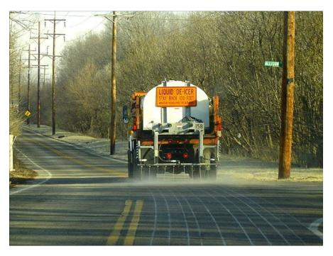
Figure 4: Department of Transportation truck sprays calcium chloride on an arterial road in Wake County, NC prior to an impending winter storm.
