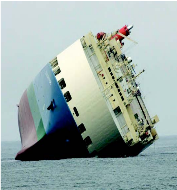
Failure to properly maintain ballast water can have catastrophic results. Ships have broken in two and/or capsized at sea when ballasting has been conducted improperly for the operational circumstances (Photo credit: Mid Atlantic Panel on Aquatic Invasive Species).
