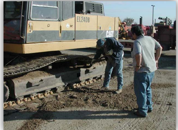
Cleaning heavy accumulations of mud prior to inspect may reveal covered or trapped invasive species (Photo credit: Bureau of Reclamation)
