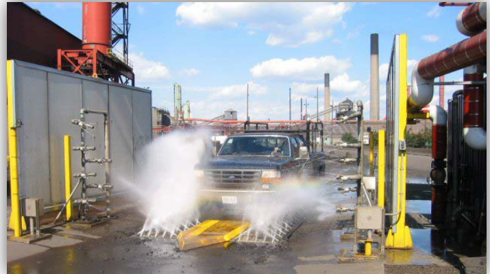
Identifying a facility to properly wash vehicles and equipment is an important step in the prevention of invasive species (Photo credit: Bureau of Reclamation).
