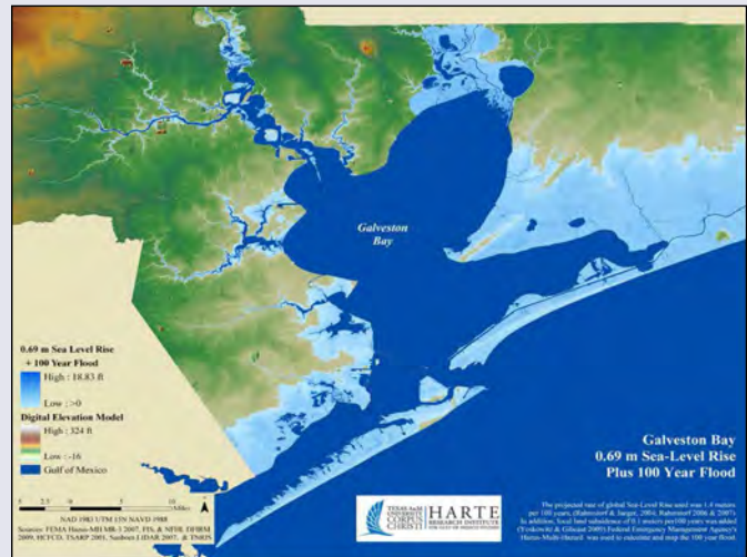
Figure 10. Land inundation given a 0.69 meter rise in sea level and a 100-year flood. Source: Yoskowitz et al., 2009.
