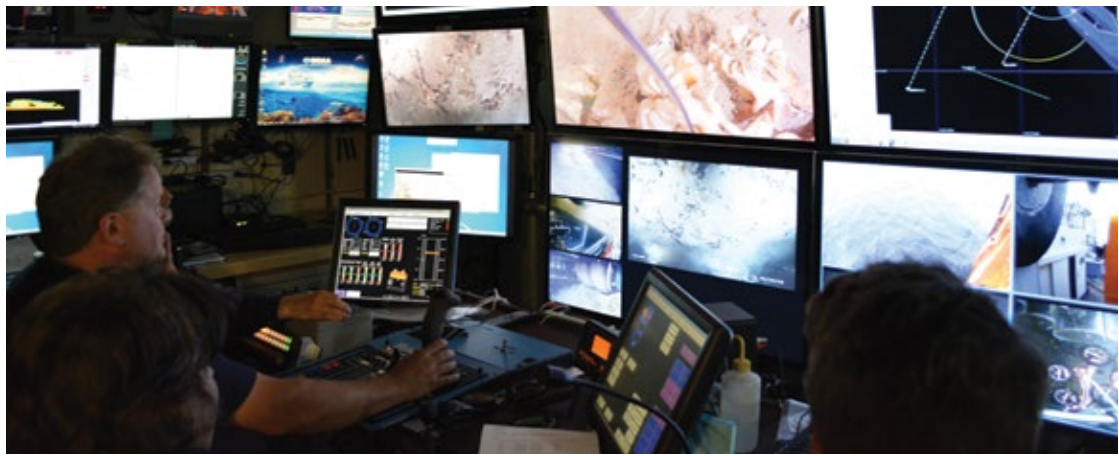
Control room for the Canadian ROPOS remotely operated vehicle.
