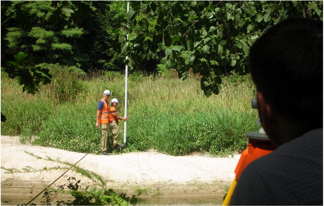
Measuring elevation and distance on a transect.
