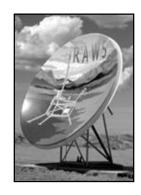
The hourly weather information collected by the RAWS is transmitted through a satellite, back to NIFC, and then distrbuted to varous locations via the internet.
