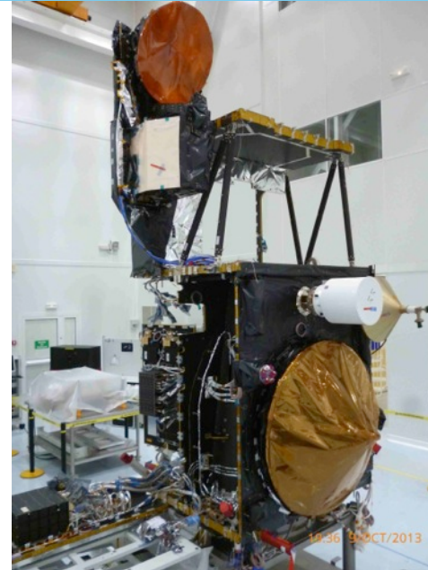
S3A Satellite at TAS-F, Cannes with Topo P/L installed
