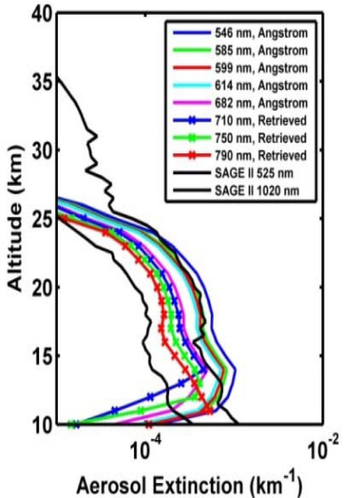
Expected performance of OMPS Limb Profiler ozone and aerosol profiles versus SAGE II.
