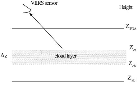
Figure 1. Overview of the methodology used to retrieve the Cloud Base Height EDR from VIIRS data.
