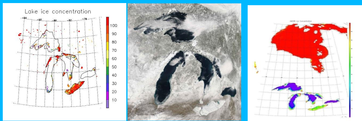
Figure 7. Lake ice concentration (%) with MODIS Aqua data (left, MODIS true color image (middle), and ice concentration from AMSR-E (right) over Great Lakes on February 24, 2008.
