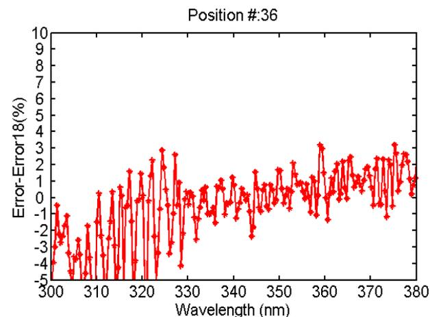
The biases at far wing positions (1-4 and 33-36) are out of specifications at wavelengths less than 320 nm. The causes can be related to complex RT processes, etc.
