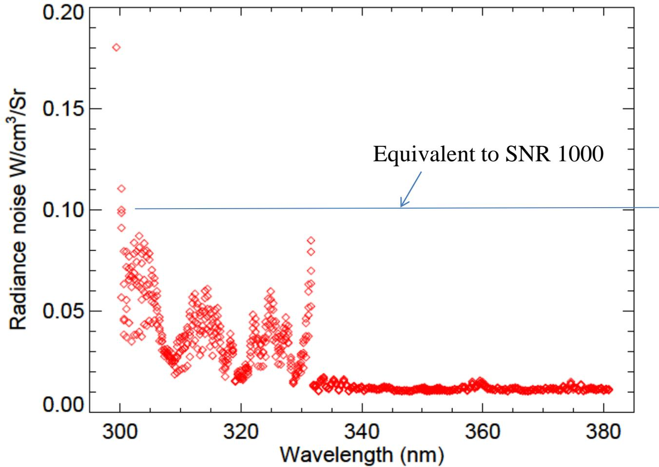
Sensor signal to noise ratio from EV data meets the requirement of 1000.
