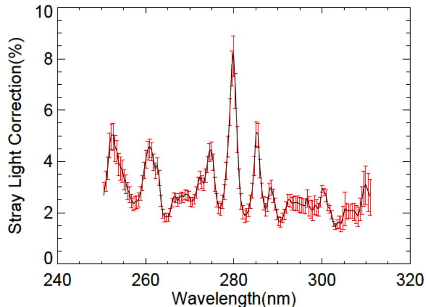
Example of orbital stray light correction vs. prelaunch predicted value shows that the orbital stray light correction is adequate across all the wavelengths
