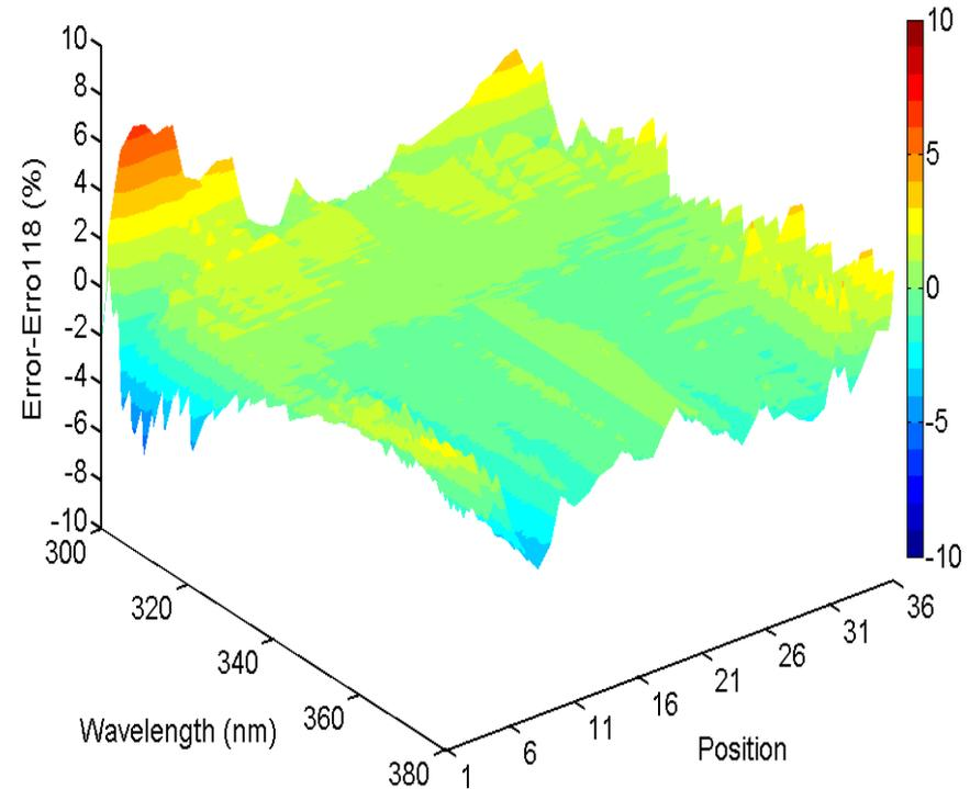
The bias in cross-track direction is generally less than 2% except at shorter wavelengths where simulations may become less accurate due to complex scattering process. The bias is also larger in side pixel locations
