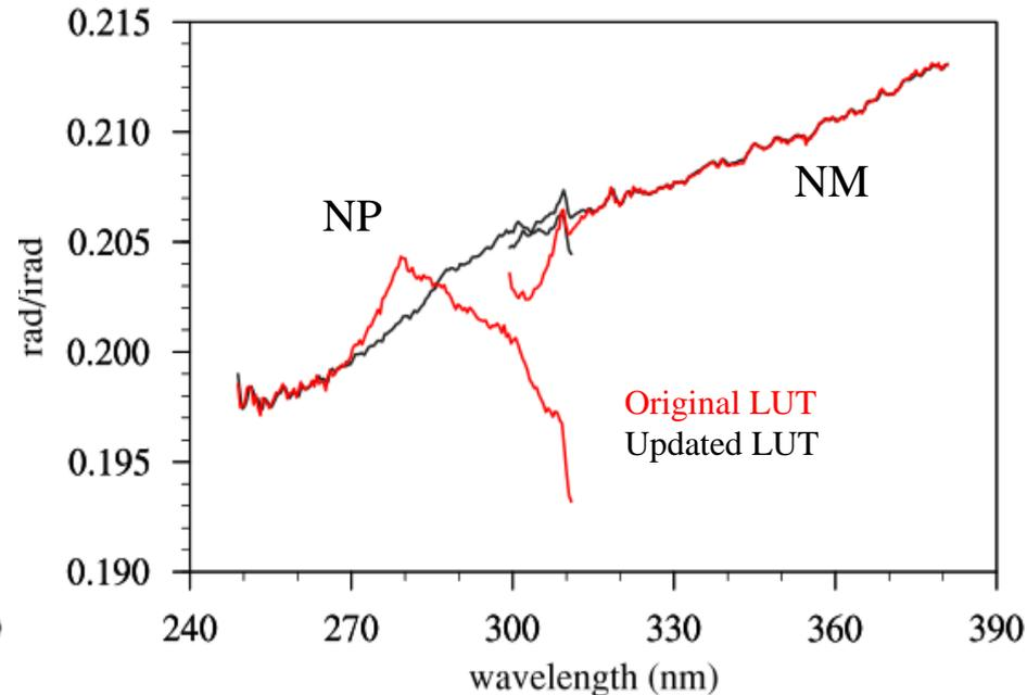
Updated radiance coefficient LUTs improve normalized radiance consistency up to ~10% between NP and NM in 300-310 nm.
