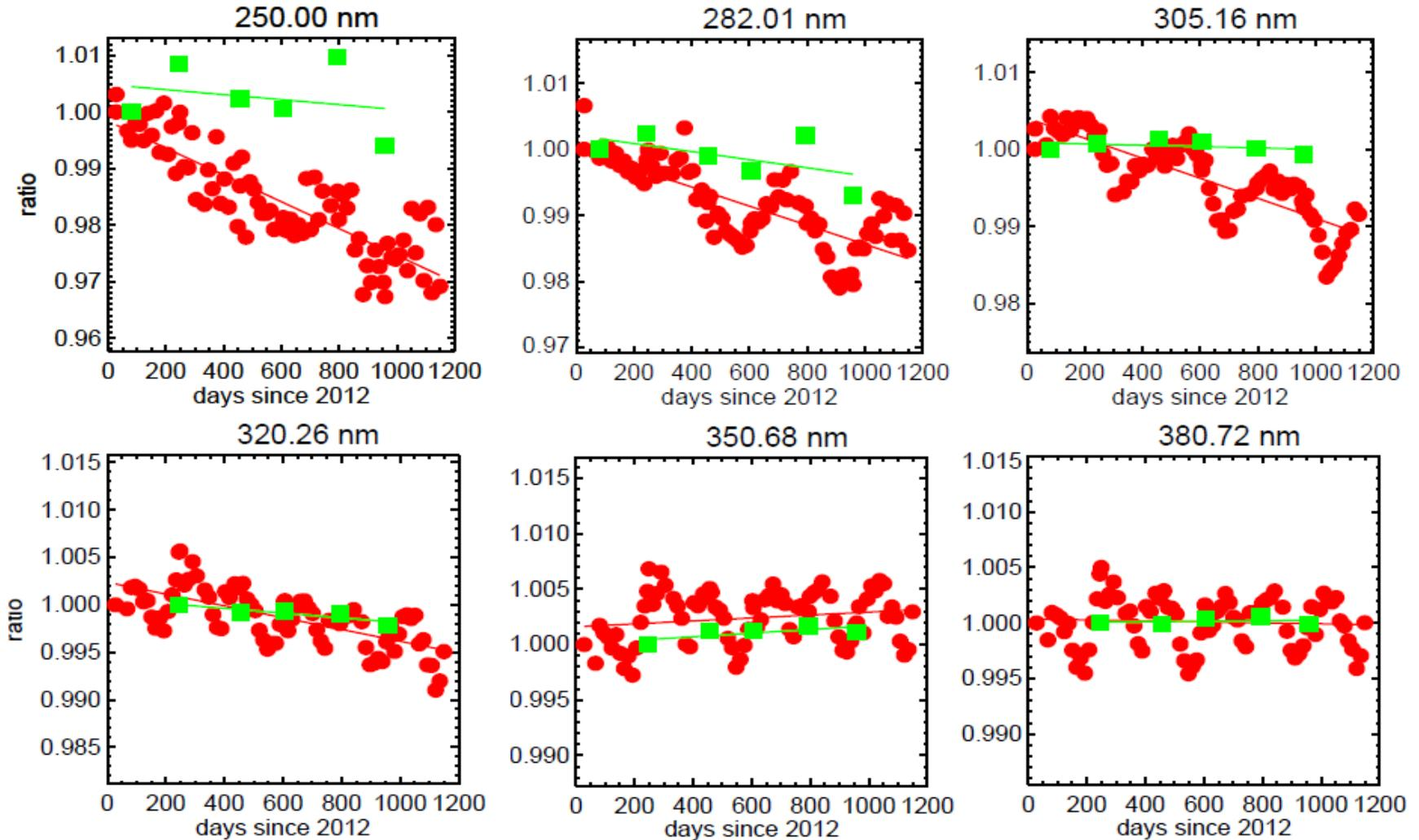
Sensor optical degradation < 1.0 %.
