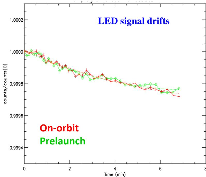
Observed OMPS TC LED drifts over time meets the system requirement of  $< 1\%$  per minute
