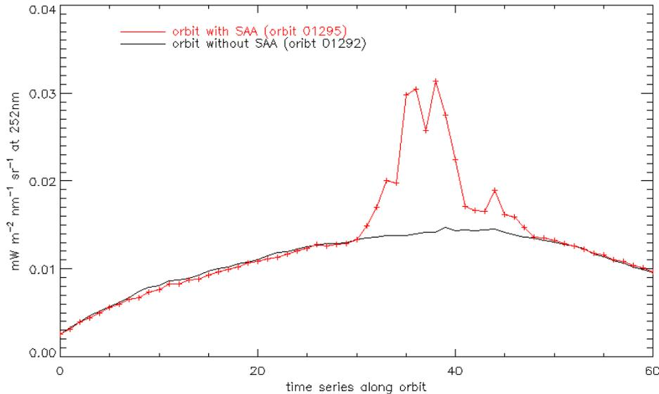
The noise/spikes show the expected increases when an orbital path falls within the SAA but return to normal levels after passing through it.
