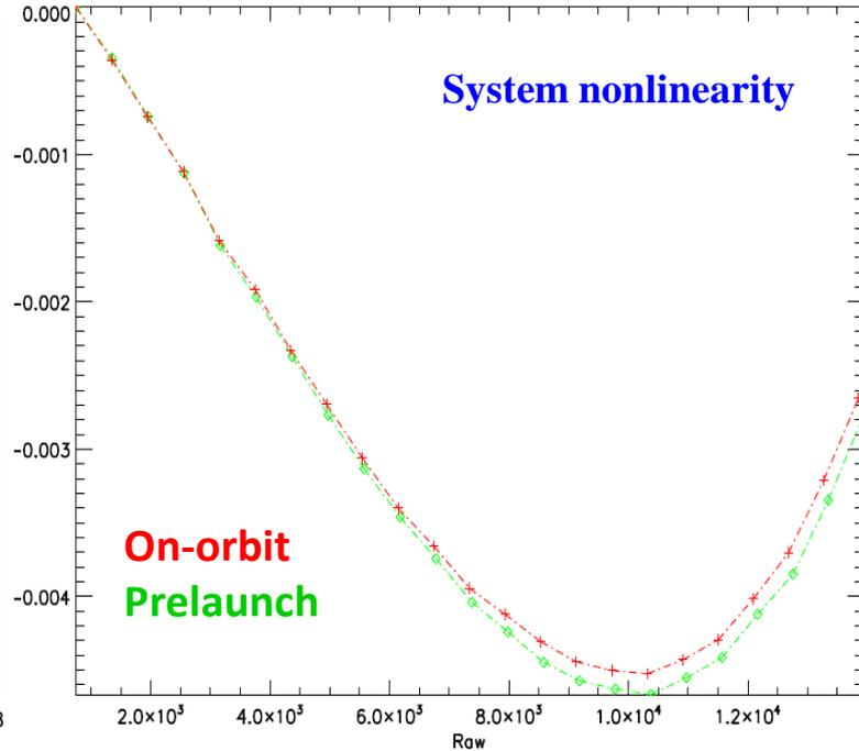
Sensor nonlinearity is compliant with the specification of  $< 2\%$
