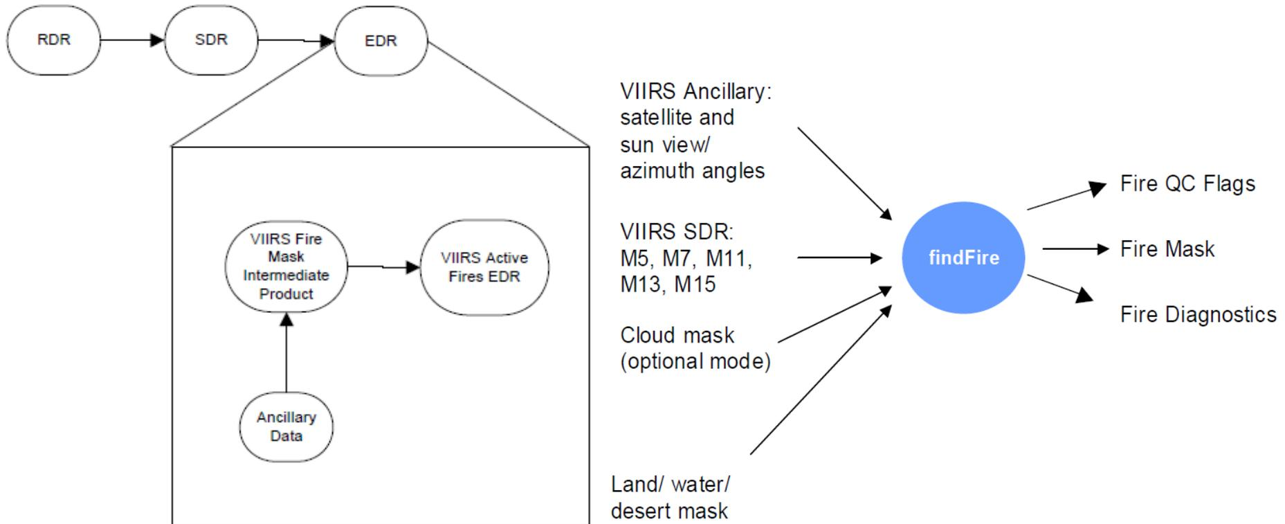
OAD VIIRS Active Fires 474-00064 January 18, 2012; Figure 1 (Processing Chain Associated with VIIRS Active Fires ARP)
