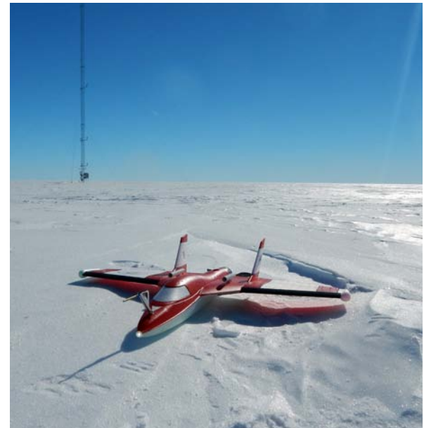
Small unmanned meteorological observer and the 30-meter tall tower automatic weather station on the Ross Ice Shelf, Antarctica.
