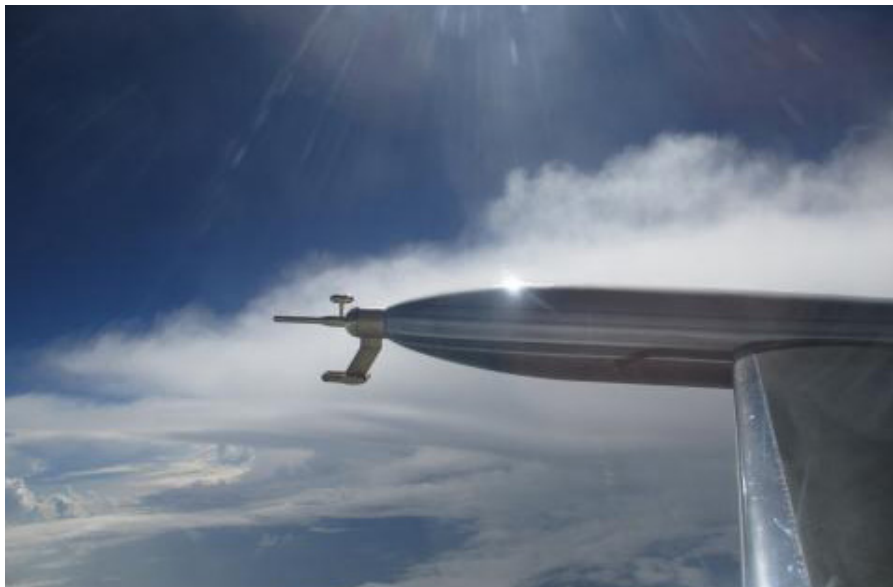
SEAC4RS Mission's SPEC Lear jet with starboard wingtip instrumentation.
