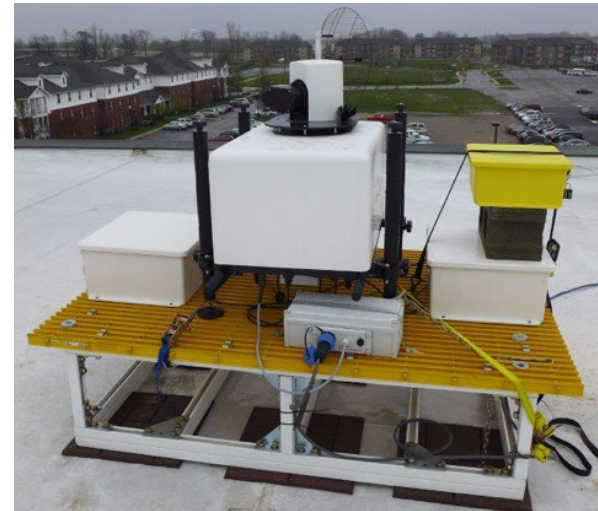
Compact Doppler lidar deployed on the roof at Ivy Tech Community College outside Indianapolis. The lidar steps through a series of conical and vertical scans and an interval of vertical staring to provide profiles of wind speed and direction, horizontal and vertical velocity variance, and aerosol backscatter signal strength three times per hour. Photo credit: Scott Sandberg/NOAA
