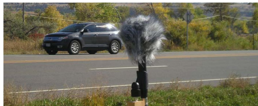
Measuring wind with microphones as a car zooms by on the Diagonal Highway, Boulder, Colorado. Photo credit: Mikhail Charnotskii/ZelTech and NOAA
