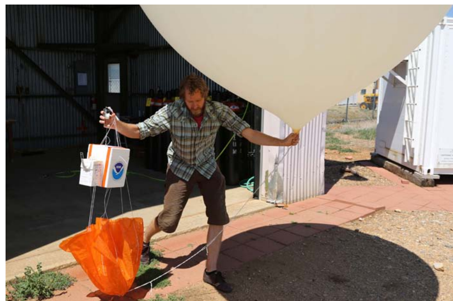
CIRES' Patrick Cullis releases a high-altitude balloon, which carries ozone-measurement equipment up to 20 miles high in the atmosphere, from a monitoring site in Boulder, Colorado. Photo credit: David Oonk/CIRES
