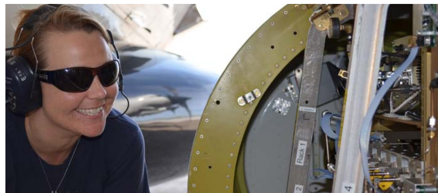
Researcher Jessica Gilman (CIRES and NOAA) next to the whole air samplers aboard the NOAA WP-3D aircraft. Each sampler holds a “snapshot” of ambient air collected every few minutes during a research flight. Each gas sample is then analyzed for hundreds of different compounds back on the ground.
