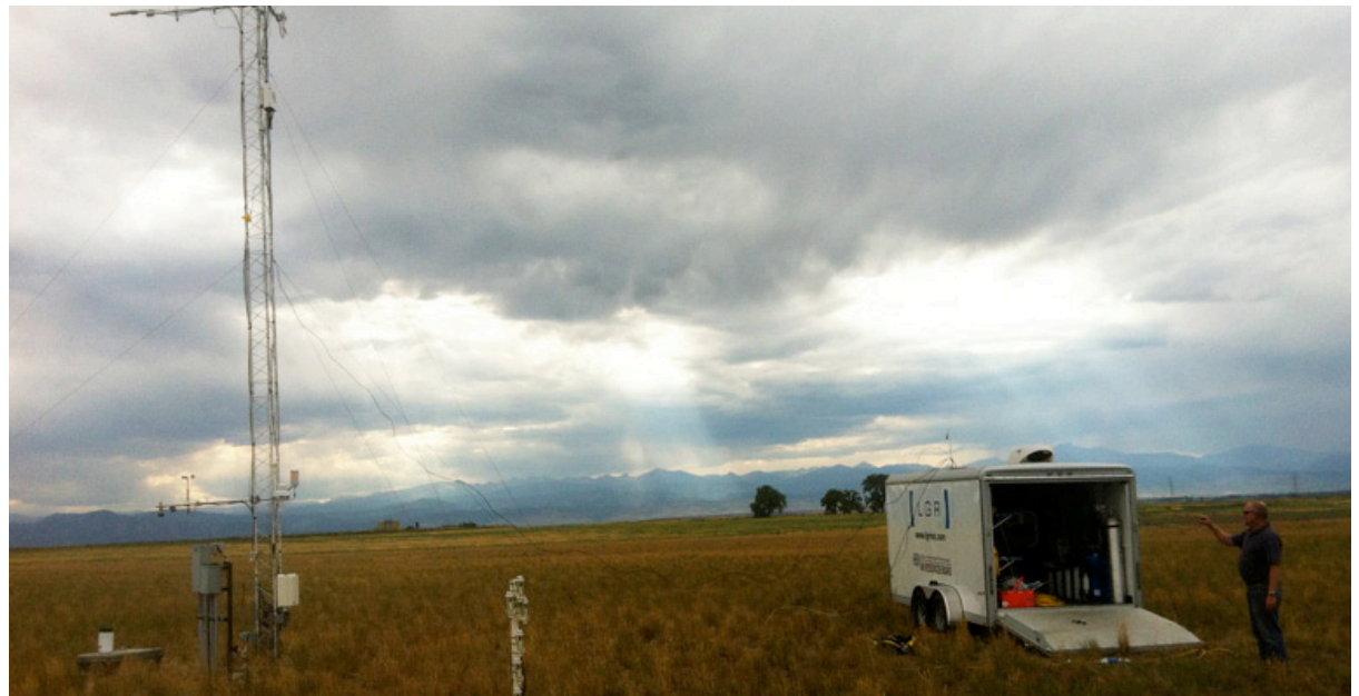
Making measurements of CO 2 and COS at the Boulder Atmospheric Observatory tall tower site operated by NOAA. Measurements were made by drawing sample air into a mobile laboratory fitted with gas analyzers and calibration equipment. Photo courtesy of David Noone/CIRES
