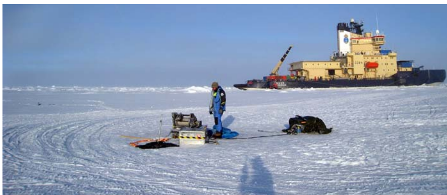
Researchers atop Arctic sea ice will measure cloud and atmosphere properties by using a tethered balloon during the Arctic Summer Cloud Ocean Study.
