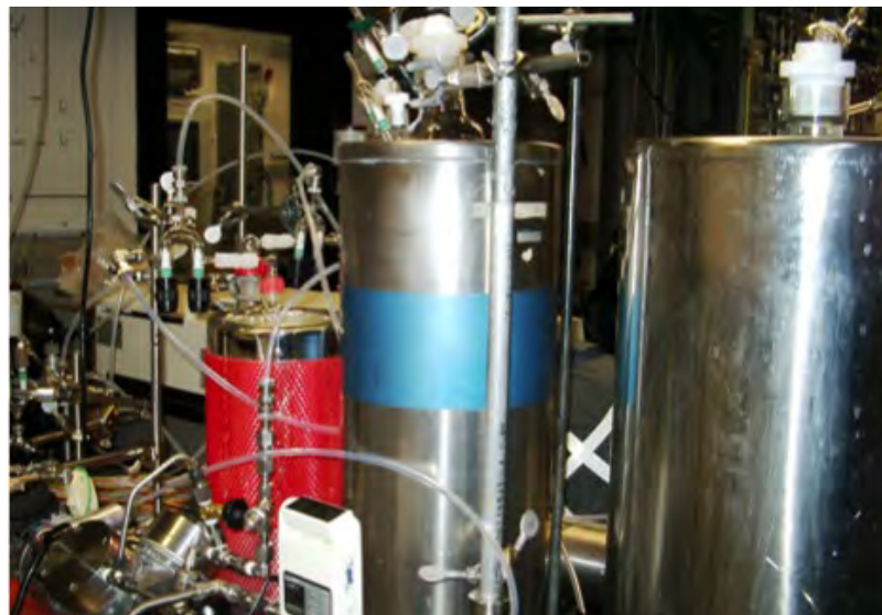
Laboratory apparatus used to study solubility and hydrolysis
