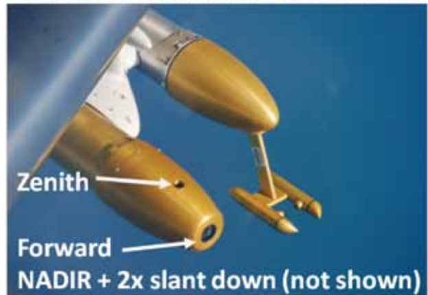
Figure 1: Pylon mounted below the wing contains sensors that measure glyoxal, iodine oxide, bromine oxide, nitrogen dioxide, formaldehyde, and other gases.
