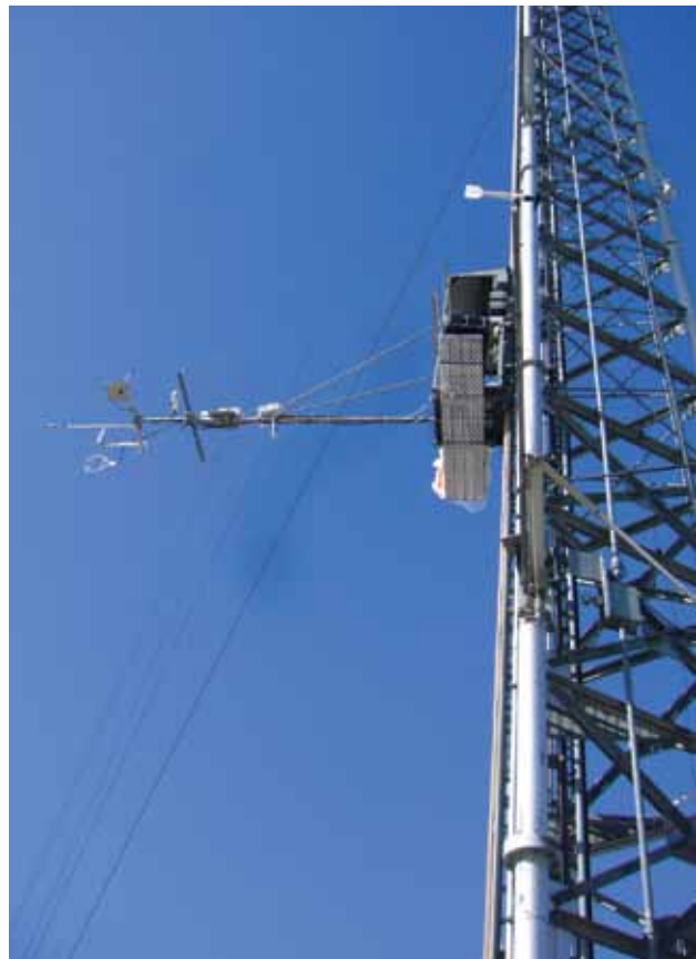
Figure 2: The instrument package on the elevator ascending the 300-m NOAA Boulder Atmospheric Observatory tower.
