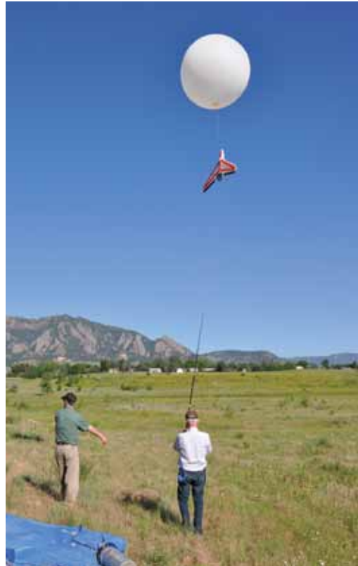
Figure 1: The Stryker suspended below a conventional meteorological balloon, a technique that will be employed for high-altitude measurements.
