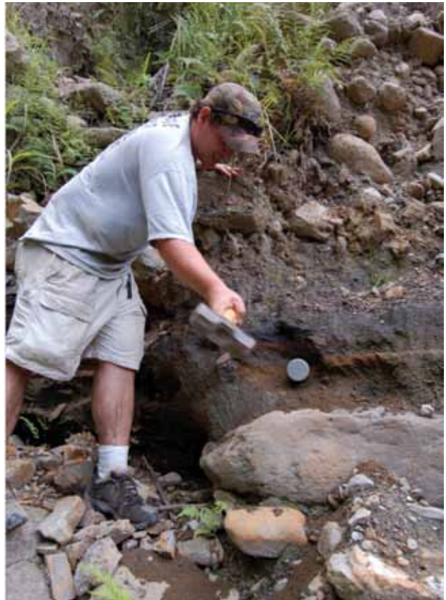
Brian Yanites collects a sample for optically stimulated luminescence dating by pounding a hollow tube into a fluvial sand deposit.
