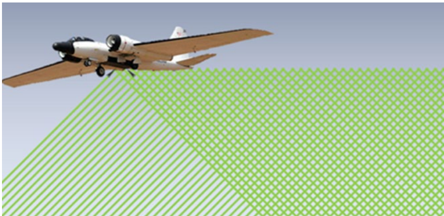
Diagram showing the scan pattern for deployment of a wind lidar on the NASA WB-57 aircraft to test the feasibility of measuring winds from a space platform. Ball Aerospace
