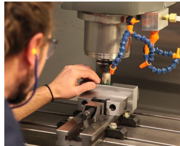
Danny Warren setting up a CNC to machine the part designed above.
