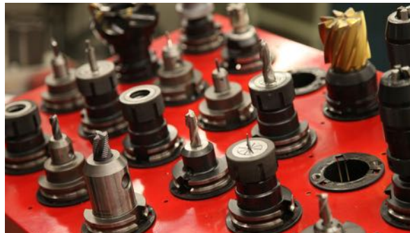
Tooling for Computer Numerically Controlled (CNC) milling machine.
