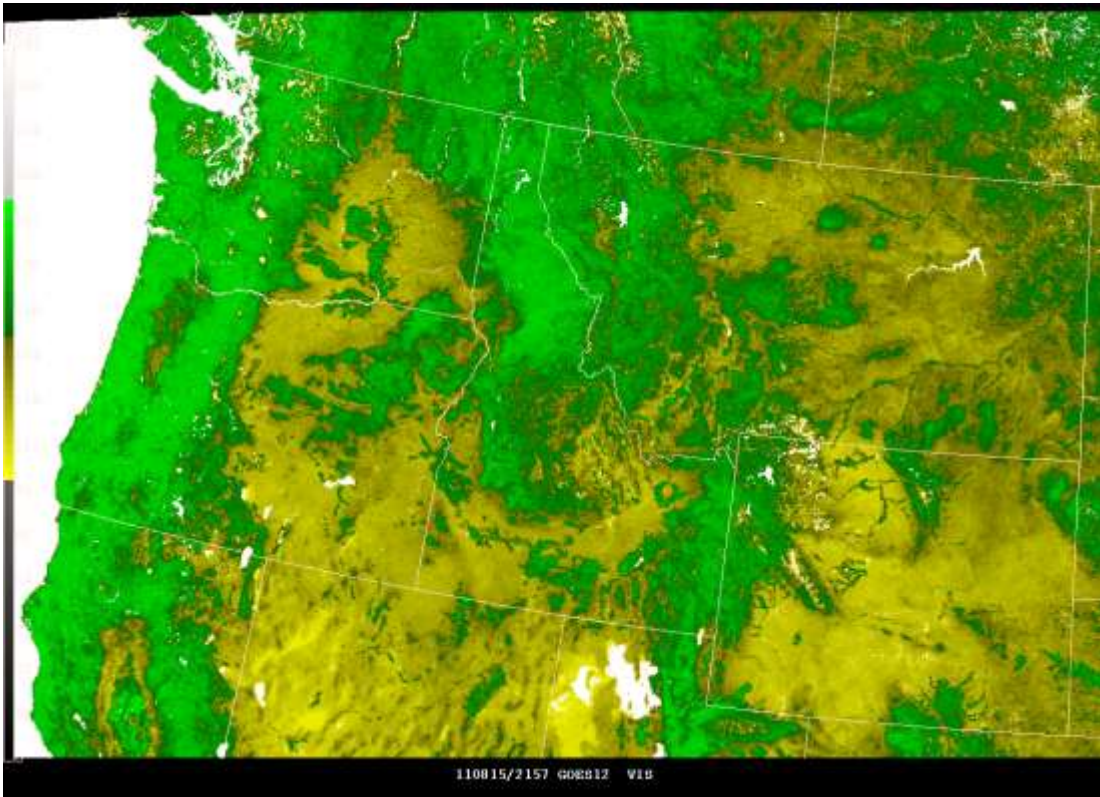
Figure 4 – Example 14-day NDVI composite displayed within HWT N-AWIPS workstations. Areas of green indicate green vegetation, whereas areas of yellow indicate regions of dead, dry or no vegetation. Areas of white indicate regions indicate missing data due to areas of water or cloud cover.
