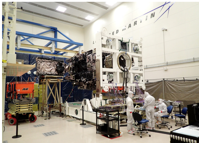
GOES-R in electromagnetic interference test configuration. Credit: Lockheed Martin
