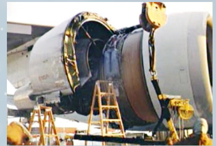
KLM passenger jet engine damaged by volcanic ash
