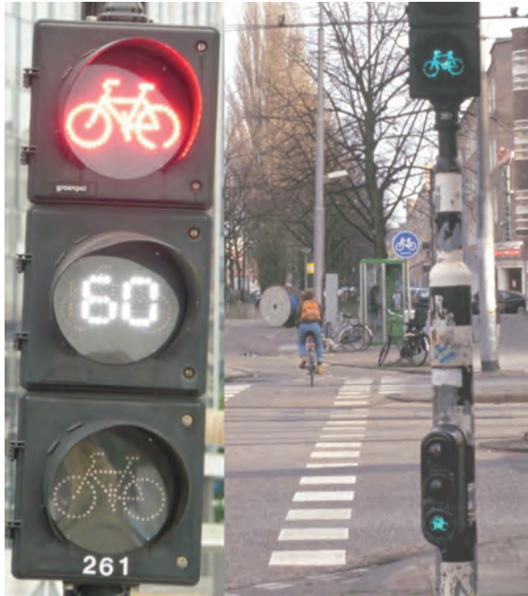
Special Traffic signals give cyclists priority and display seconds till green light.
