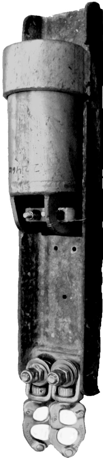
Figure 2F. - - Photo of the bottom contact sensor and its attachment configuration to the ground gear used during the 2008 EBSS survey.
